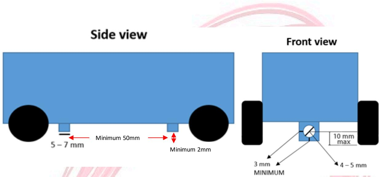
The diagram above shows the dimension ranges for the eyelets as stated in rule 9.
